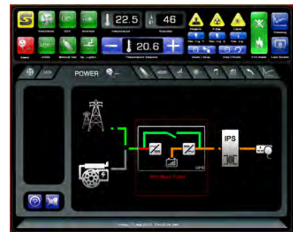
UPS Mains Failed – On Battery
