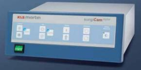
The surgiCam® control unit allows manual as well as automatic control of all camera functions.
