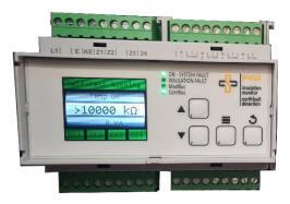
The IPM has several additional features such as included search current generator for failure location detection (additional device for localisation required), one change over relay contact, two NO-Solid-State-Relays contacts, four digital inputs, transformer load monitoring, transformer temperature monitoring, one RS485 with Modbus Protocol for reading device measurement values and alarms and one RS485 to communicate with fault localisation devices.
