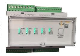
Only useable in combination with an IPM. Communication between the IPM and the EDS is via an RS485 interface. Maximum 5 devices can be connected to one insulation monitor. The device has 20 LEDs to show its system status.
