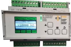
The IPM has several additional features like included search current generator for failure location detection (additional device for localisation required), one change over relay contact, two NO-Solid-State-Relays contacts, four digital inputs, transformer load monitoring, transformer temperature monitoring, one RS485 with ModBus-Protocol for reading device measurement values and alarms and one RS485 to communicate with fault localisation devices.
