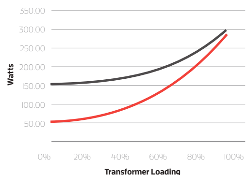
10 kVA Standard Transformer - Heat Losses
