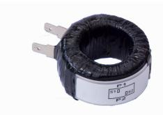
This product is a current transformer, which is used to measure the load which in applied to an IPS transformer. It is installed within the IPS panel and has 1 leg of the secondary side of the transformer run through it. The winding relationship allows for a voltage to be derived on the output terminals when current is drawn though the primary, this voltage is seen by the IPM400/EDS400 unit which enables the monitoring device to determine what load is being applied.
